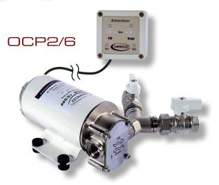
Oil change systems. The operative functions of the pump are electronically controlled by a membrane panel. The pump is equipped with 1 or 2 valves. Conceived for oil fill and drain operations. The electronic card adjusts the speed of the pump according to oil viscosity/temperature. It also increases the speed of the pump during priming. The system automatically shuts off in case of empty tank, short circuit and after 30 minutes of operation.
