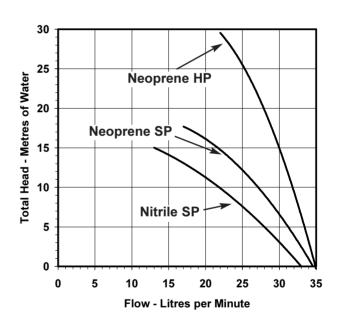
**Note**: Performance shown is for a new pump, pumping water at 20°C, performance may vary by up to 15%. Consult factory for performance of alternative impeller compounds.
