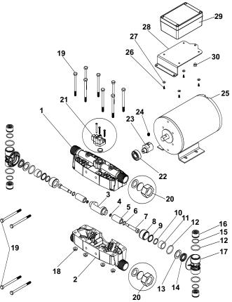
NOTE: When ordering parts, give QUANTITY, PART NUMBER, DESCRIPTION, and COMPLETE PUMP MODEL NUMBER. Reference numbers are used ONLY to identify parts in the drawing and are NOT to be used as order numbers.
