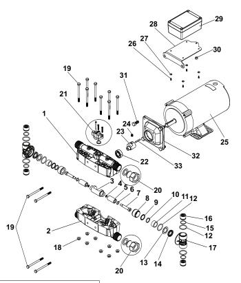
NOTE: When ordering parts, give QUANTITY, PART NUMBER, DESCRIPTION, and COMPLETE PUMP MODEL NUMBER. Reference numbers are used ONLY to identify parts in the drawing and are NOT to be used as order numbers.
