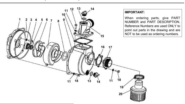
Standard Seal Kit No. 3430-0799 Consists of (1) Ref. 2 O-ring, (4) Ref. 3 Sealed Washers, (1) Ref. 5 Mechanical Seal, (1) Ref. 8 O-ring, (1) Ref. 10 Outlet Sealed Washer, (2) Ref. 13 O-rings, and (1) Ref. 16 Check Valve
