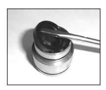
12. For all pumps (except P318/P324), use a flat screw driver to pry the oil seals (#19) loose from the seal case (#20).
