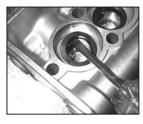
9. Remove the pressure rings (#24) and grooved seals (#23) from the valve casing (#26). Inspect parts for wear and replace if necessary. For P318 & P324 only, the spacers (#23A) can now be removed.
