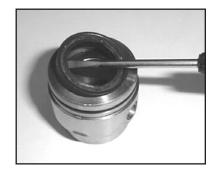
Remove the weep grooved seals (23A for all pumps except P318/P32 & #23 for P318/P324 only) from the seal case (#20).
