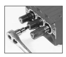
13A. P318/P324 Only! Clean the old sealant from the threads of the tension screw and the plunger base (16A). Place plunger pipes over plunger base and secure with tension screw to 220 in-lbs.
