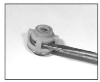
3. The valve assemblies can be separated by inserting a small screw driver between the valve seat (#27) and its valve spring retainer (#30).
