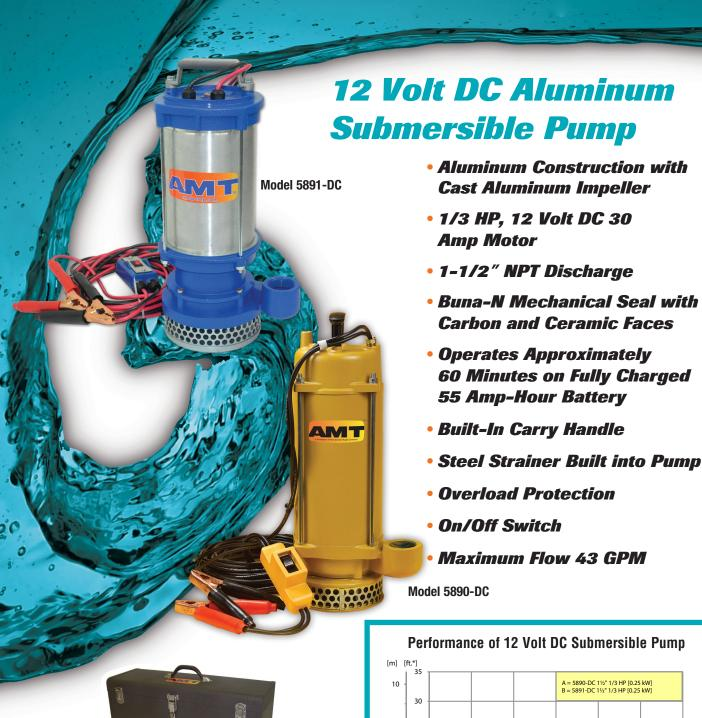
The AMT Submersible 12 Volt DC pump is designed for use in dewatering applications where limited or no electricity is present and for emergency back-up during power failure. The light weight pump is constructed of aluminum body with cast aluminum impeller. Unit comes assembled with 30 foot power cord, which has battery clips for easy attachment to 12 volt battery. Pumps are designed to handle liquids with solid content or dissolved solids and debris.
