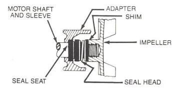
Figure 1- Mechanical Seal Replacement
